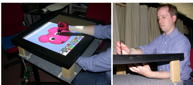
Figure 13. 3D object modeling and manipulation. Left: top-view of image being edited. Right: the user makes use of both hands simultaneously to draw and control orientation and position of the model.
