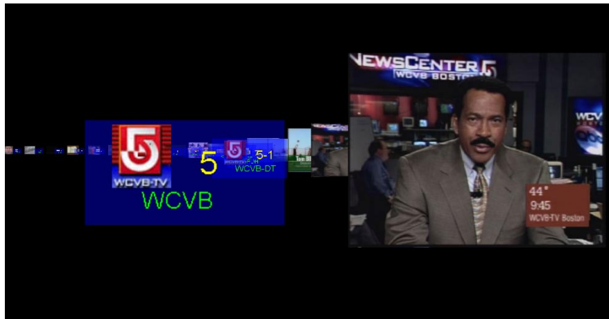
Figure 3: Screen shot of channel surfing prototype. Shown are images sampled offline for each of the channels with a second tuner.
